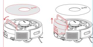
Press the red area (marked in the picture) to open bin door and empty bin.
