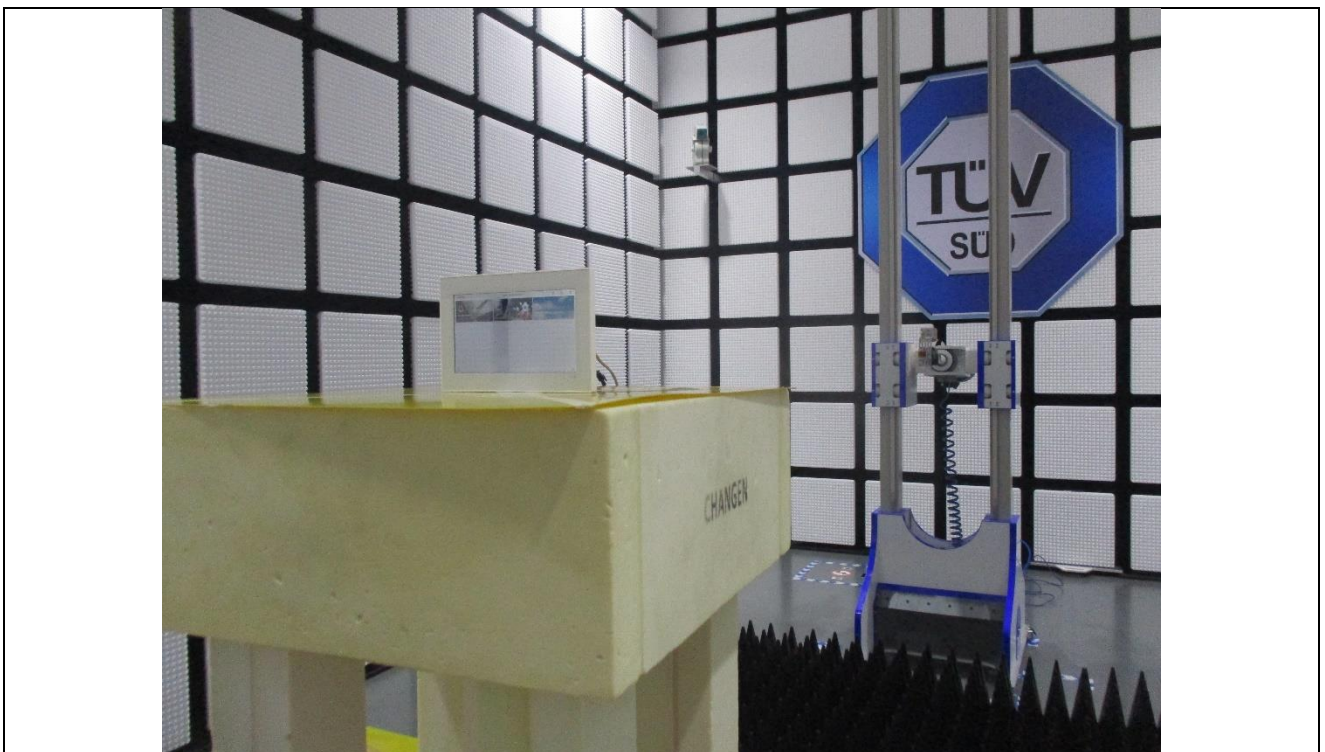
Radiated Emission test (Above 18000MHz)
