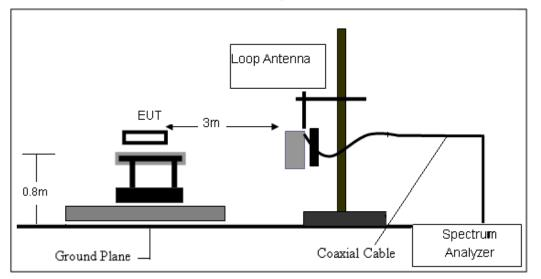
(B) Radiated Emission Test-Up Frequency 30MHz~1GHz
