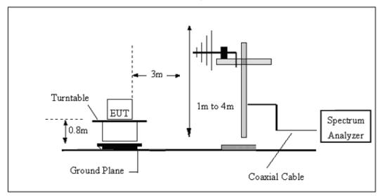
(C) Radiated Emission Test-Up Frequency Above 1GHz
