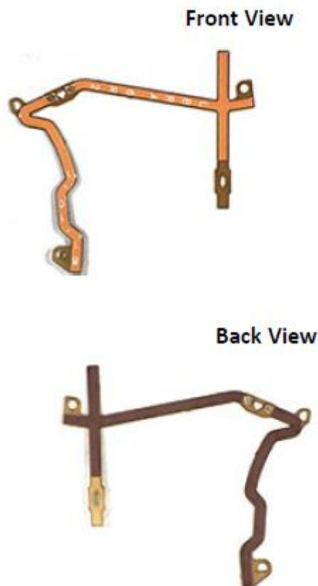
Figure 1 2.4 GHz Antenna
