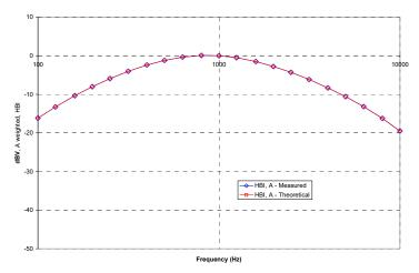
Figure 4-8 **ABM2 Frequency Response Validation**
