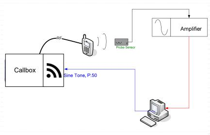
Figure 4-2 T-Coil Test Setup
