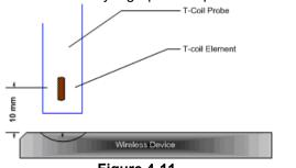
Figure 4-11 Measurement Distance
