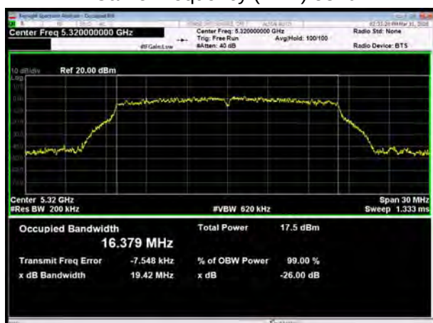
U-NII-2A, 802.11a Carrier frequency (MHz): 5320
