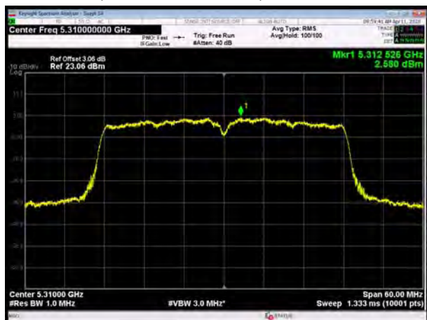
U-NII-2A, 802.11ac VHT80, Channel No.: 58
