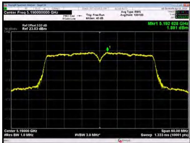
U-NII-1, 802.11ac VHT40, Channel No.: 38
