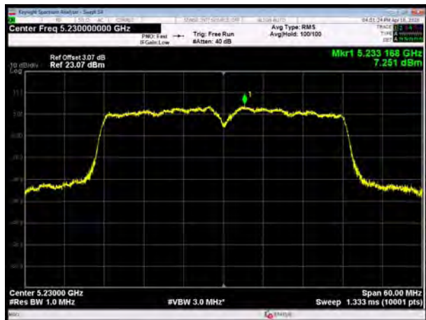
U-NII-1, 802.11ac VHT80, Channel No.: 42
