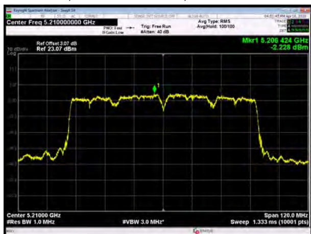
U-NII-1, 802.11ac VHT80, Channel No.: 42
