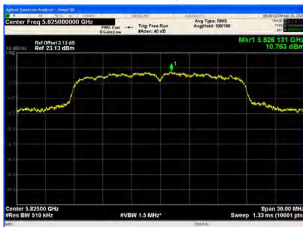
U-NII-3, 802.11ac VHT20, Channel No.: 165
