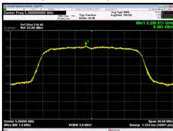
U-NII-2A, 802.11ac VHT20, Channel No.: 60
