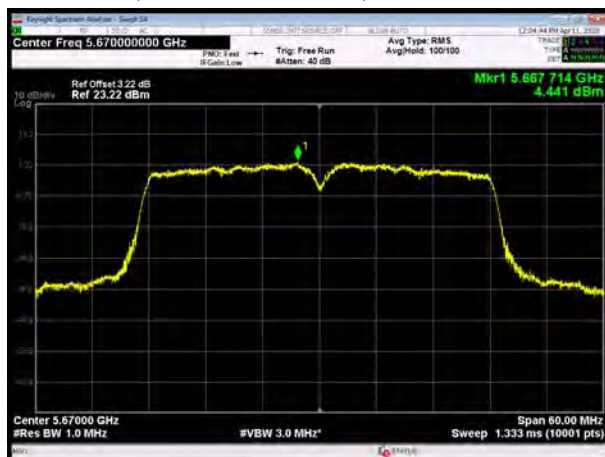
U-NII-2C, 802.11ac VHT40, Channel No.: 142
