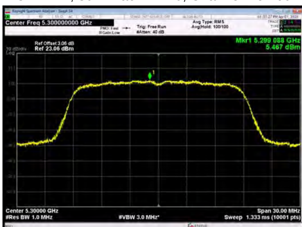
U-NII-2A, 802.11ac VHT20, Channel No.: 64
