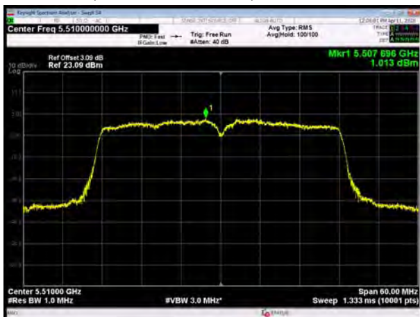
U-NII-2C, 802.11ac VHT40, Channel No.: 102
