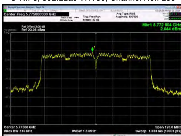
U-NII-3, 802.11ac VHT80, Channel No.: 155
