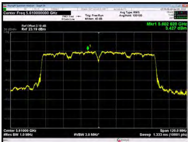
U-NII-2C, 802.11ac VHT80, Channel No.: 122
