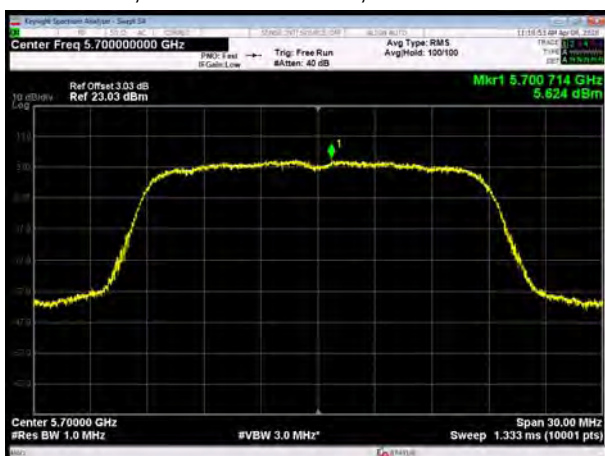
U-NII-2C, 802.11ac VHT20, Channel No.: 144
