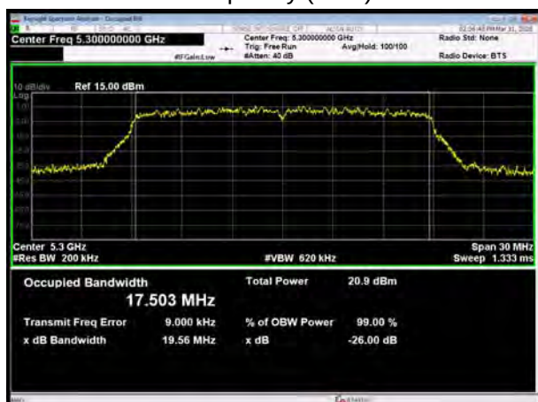
U-NII-2A, 802.11ac VHT20 Carrier frequency (MHz): 5320
