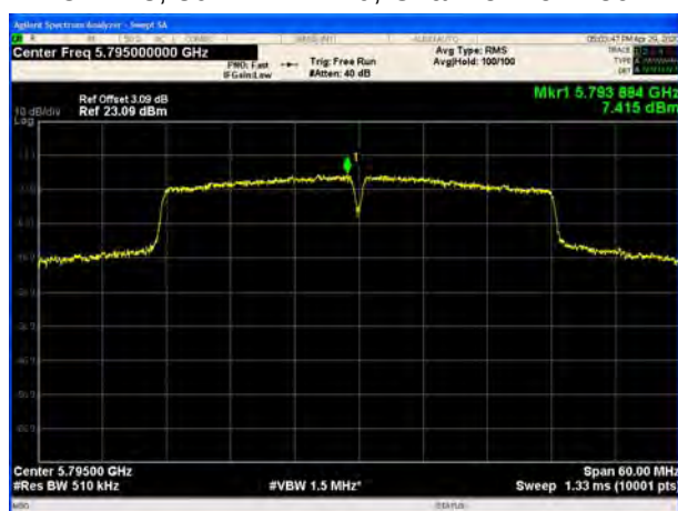
U-NII-3, 802.11ac VHT40, Channel No.: 151
