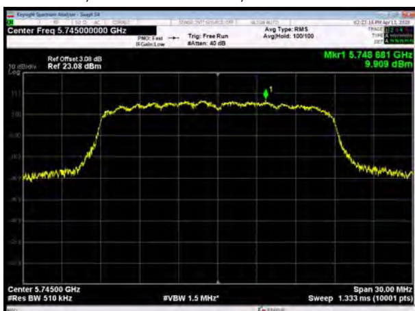
U-NII-3, 802.11ac VHT20, Channel No.: 157
