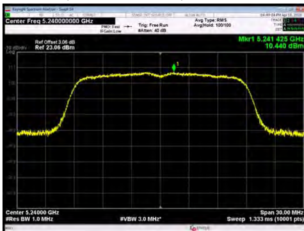
U-NII-1, 802.11ac VHT20, Channel No.: 48
