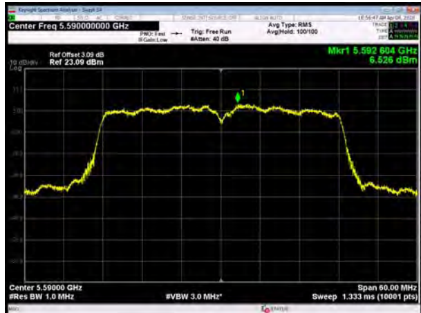
U-NII-2C, 802.11ac VHT40, Channel No.: 118
