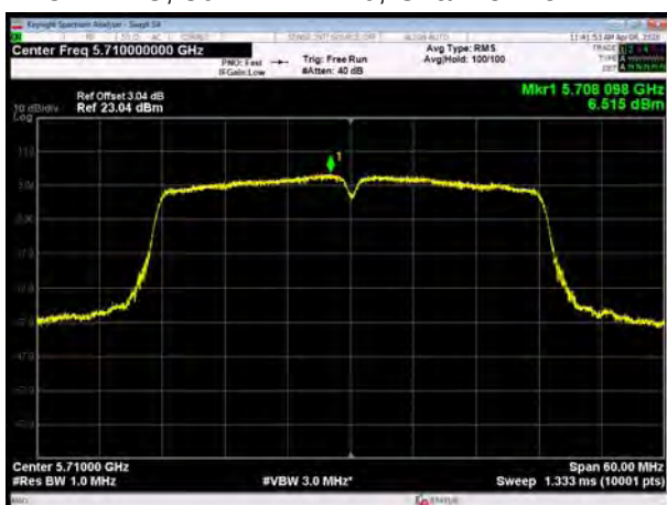
U-NII-2C, 802.11ac VHT40, Channel No.: 102
