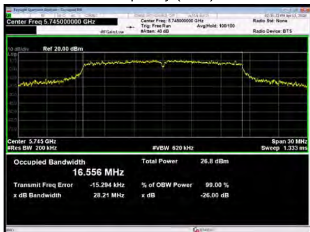
U-NII-3, 802.11a Carrier frequency (MHz): 5785
