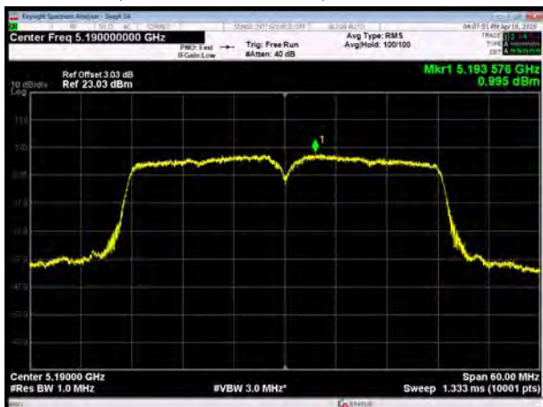
U-NII-1, 802.11ac VHT40, Channel No.: 38
