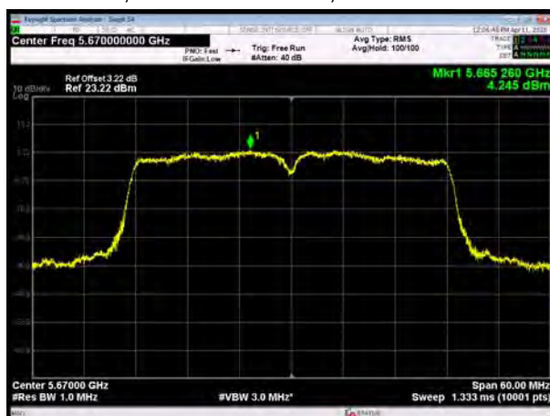
U-NII-2C, 802.11ac VHT40, Channel No.: 142
