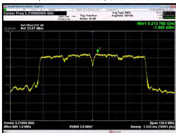
U-NII-1, 802.11ac VHT80, Channel No.: 42
