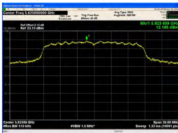
U-NII-3, 802.11ac VHT20, Channel No.: 165
