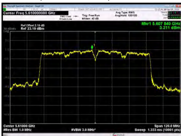
U-NII-2C, 802.11ac VHT80, Channel No.: 122
