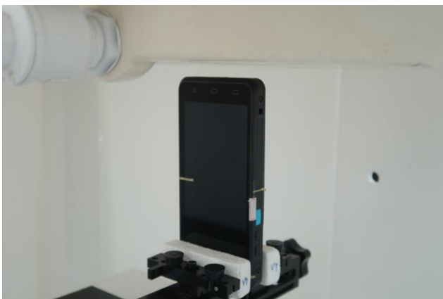
Bottom Side, Test Separation 10 mm
