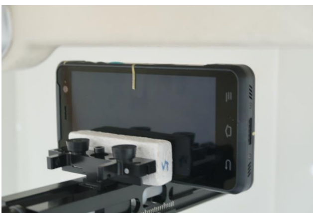
Right Side, Test Separation 10 mm
