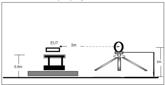
(B) Radiated Emission Test-Up Frequency 30MHz~1GHz
