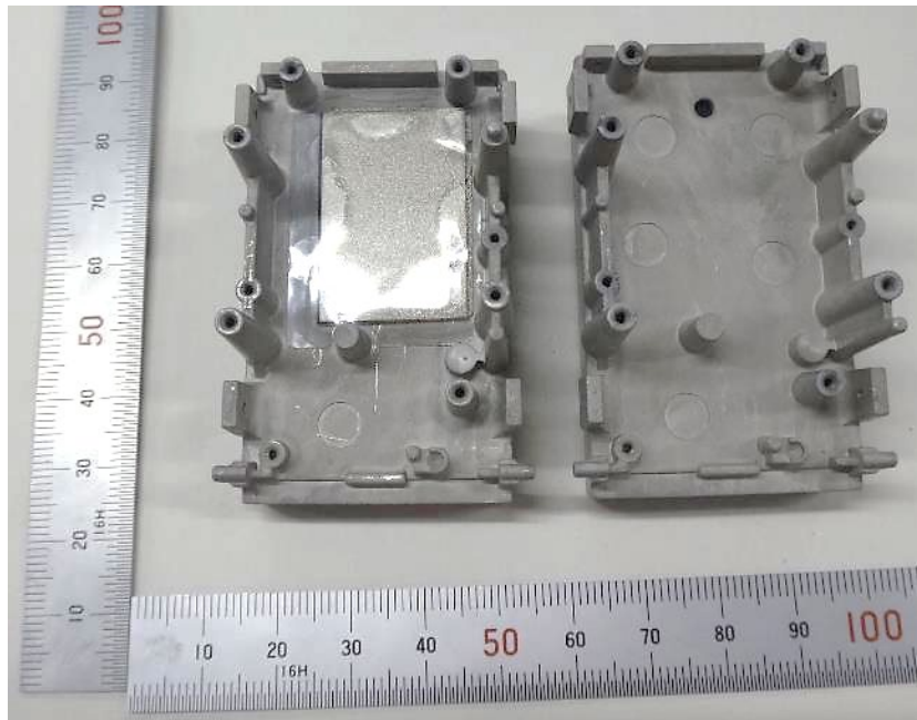
Fig.28 Remove board of RM-215
