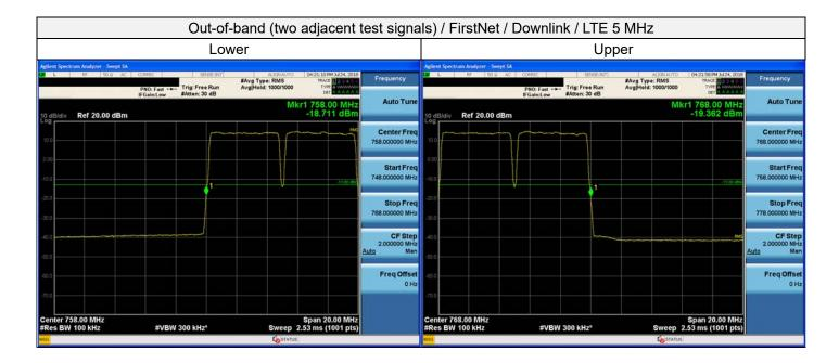
**Note:** Intermodulation test in FirstNet band are performed only for LTE 5MHz signal, because the band cannot accommodate two LTE 10MHz signals. (Refer to Section 3.6.1 of KDB 935210 D05)
