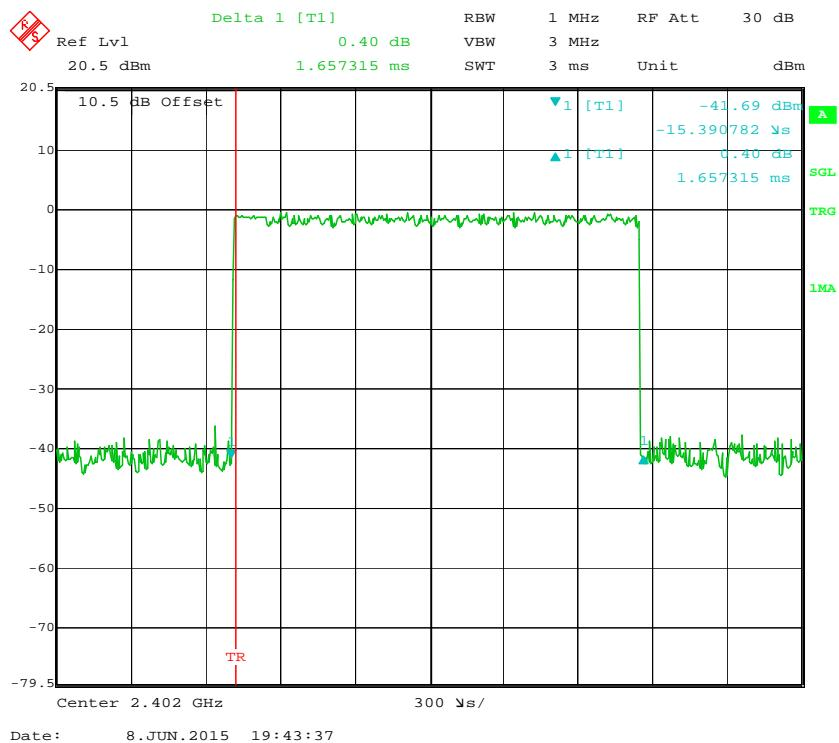
**Pulse time, Middle Channel, 3DH3**
