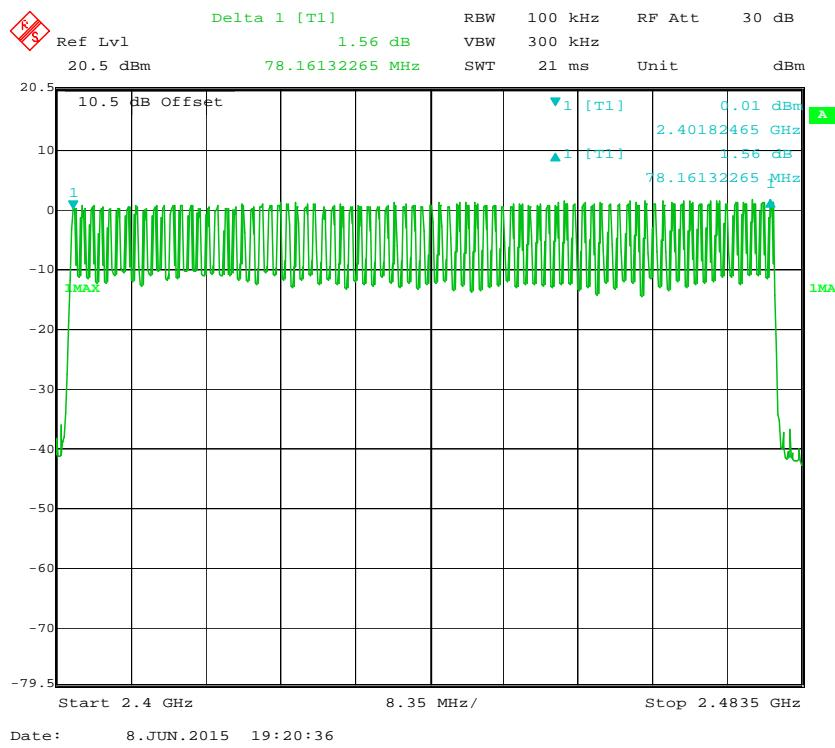
**EDR ( $\pi/4$ -DQPSK): Number of Hopping Channels**
