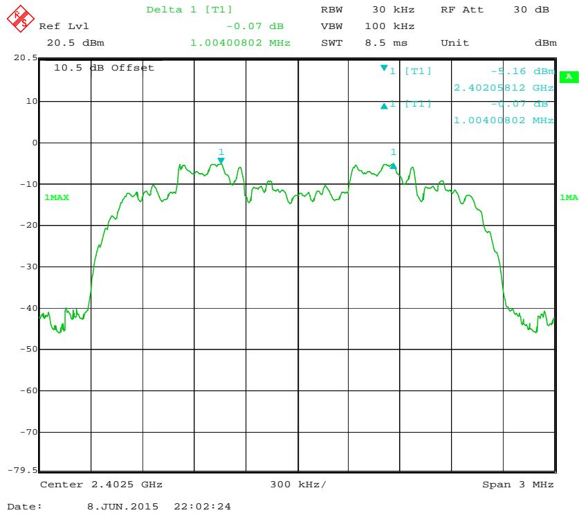
**EDR ( $\pi/4$ -DQPSK): Middle Channel**
