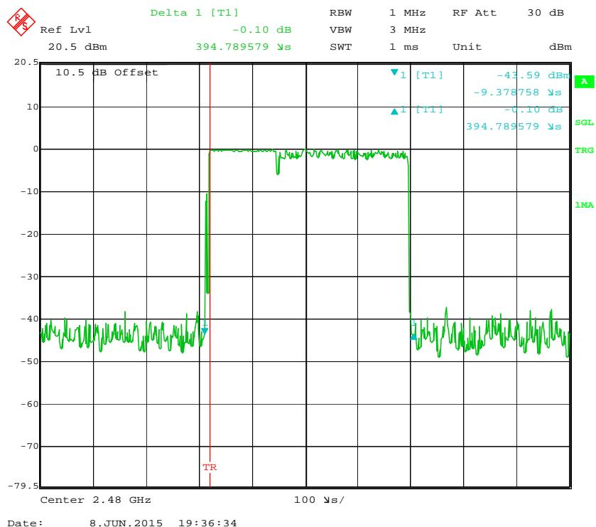
**Pulse time, Low Channel, 2DH3**
