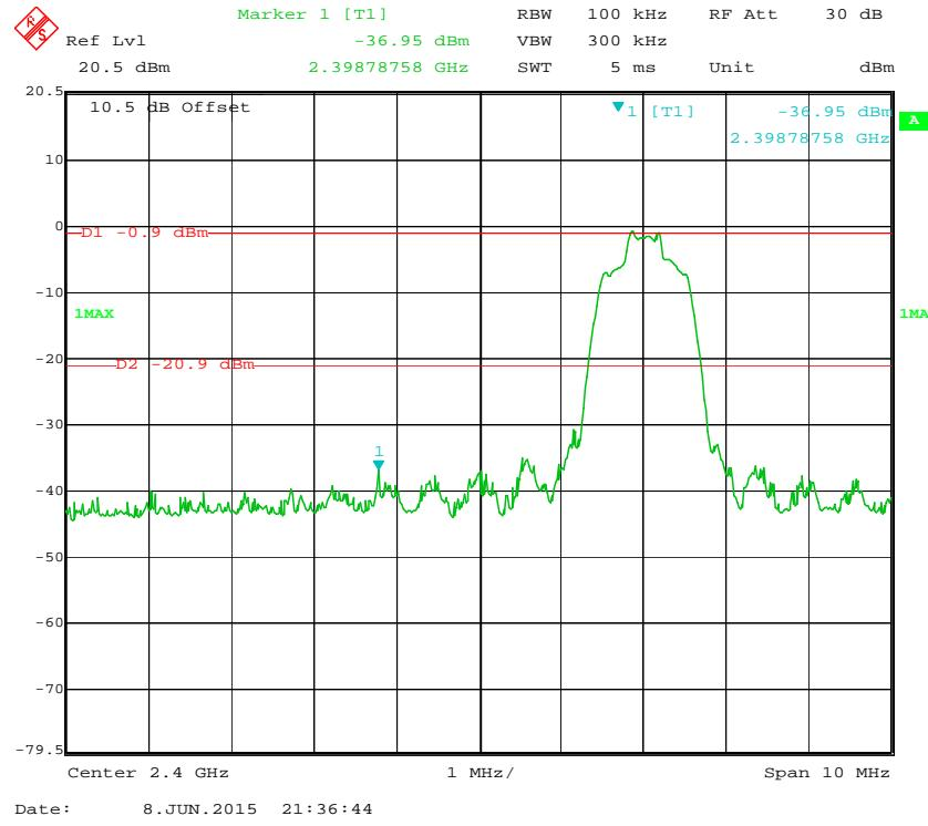
**EDR ( $\pi/4$ -DQPSK): Band Edge-Right Side**
