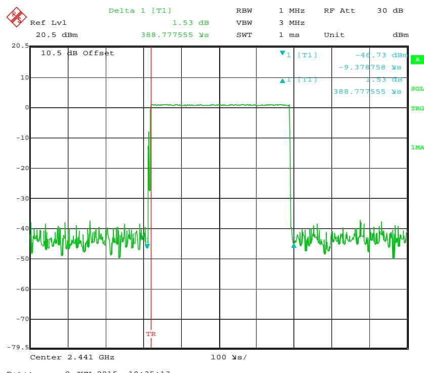
**Pulse time, High Channel, DH1**
