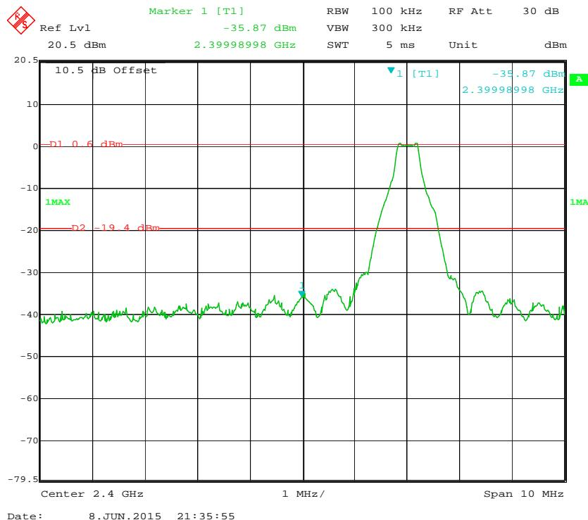
**BDR (GFSK): Band Edge-Right Side**
