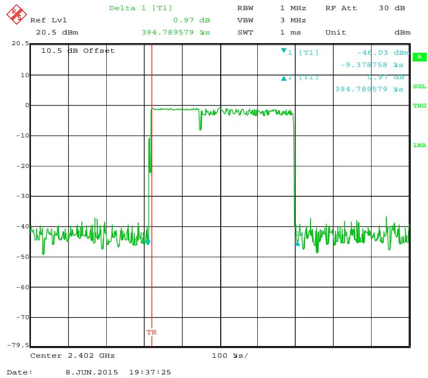
**Pulse time, Middle Channel, 2DH1**
