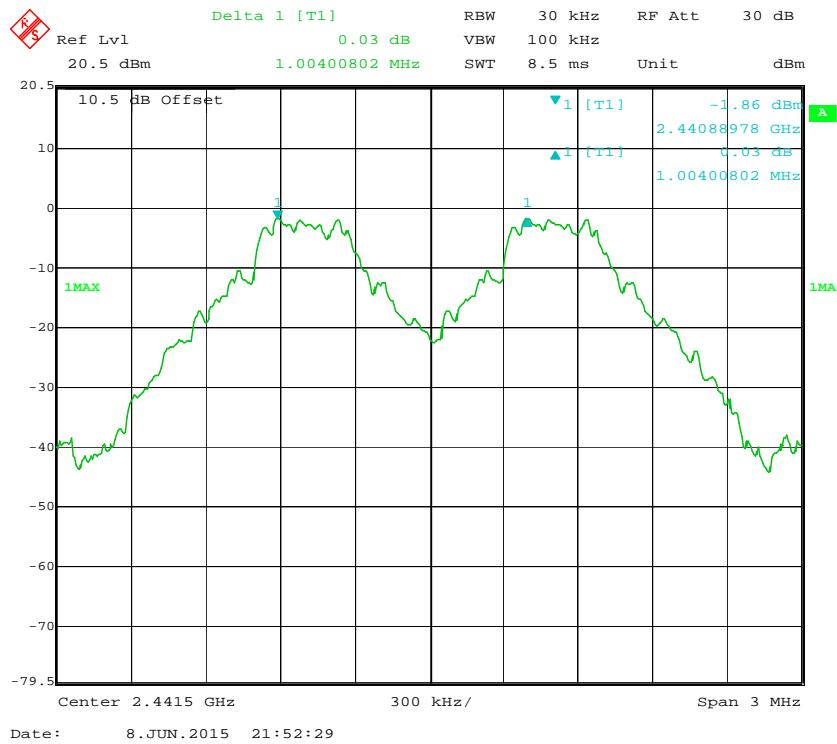
**BDR (GFSK): High Channel**
