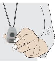
The maximum range of the Pendant from the Console is 1,000 feet under open field test conditions. Actual distance will vary with installation and environment. Pendant is not a cellular device.
