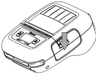
2. Load the roll paper in the orientation shown in the figure below.
