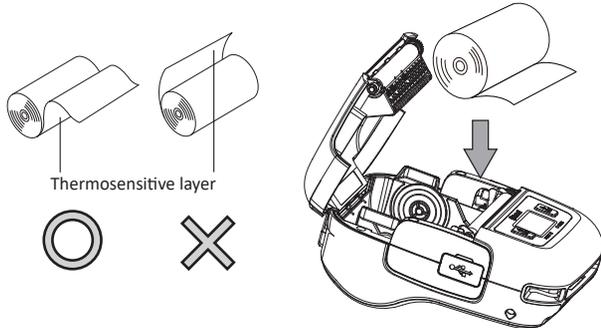
3. Pull the end of the roll straight toward you. Then press down on both sides of the printer cover to close it firmly. When you close the printer cover, make sure that it is closed on both sides.
