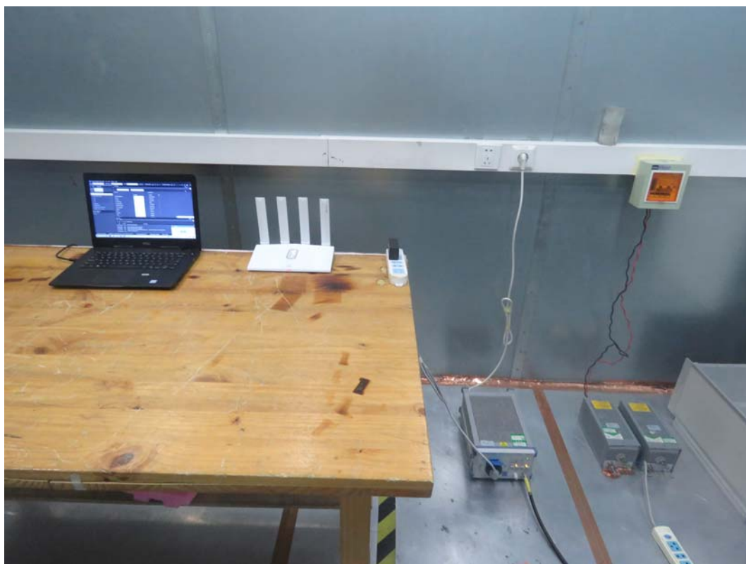
Picture 2 Conducted Emission Test Setup
