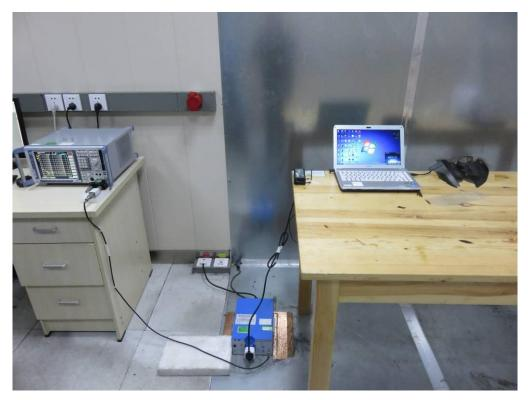
FCC RADIATED EMISSION TEST SETUP
