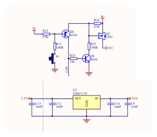
1. This part is a self-locking switch circuit. When the key is pressed, the main chip detects that the key is pressed. The main chip controls the electronic switch and supplies power to the main chip after the voltage regulator is stabilized
