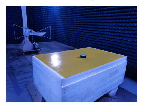
Radiated Emissions Test View (Above 1GHz)
