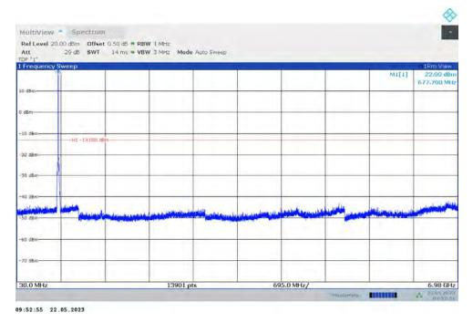
n77L NOTE: peak above the limit line is the carrier frequency.
