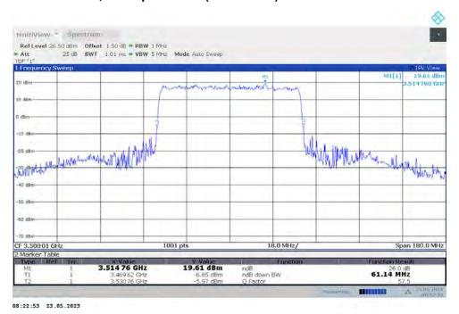
n77L,60MHz Bandwidth,DFT-s-QPSK (-26dBc BW)
