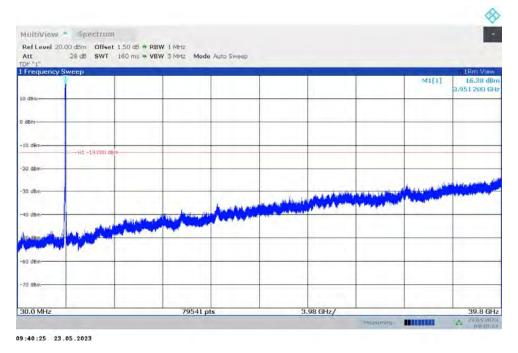
n78L NOTE: peak above the limit line is the carrier frequency.
