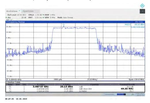
n78L,50MHz Bandwidth,DFT-s-QPSK (-26dBc BW)
