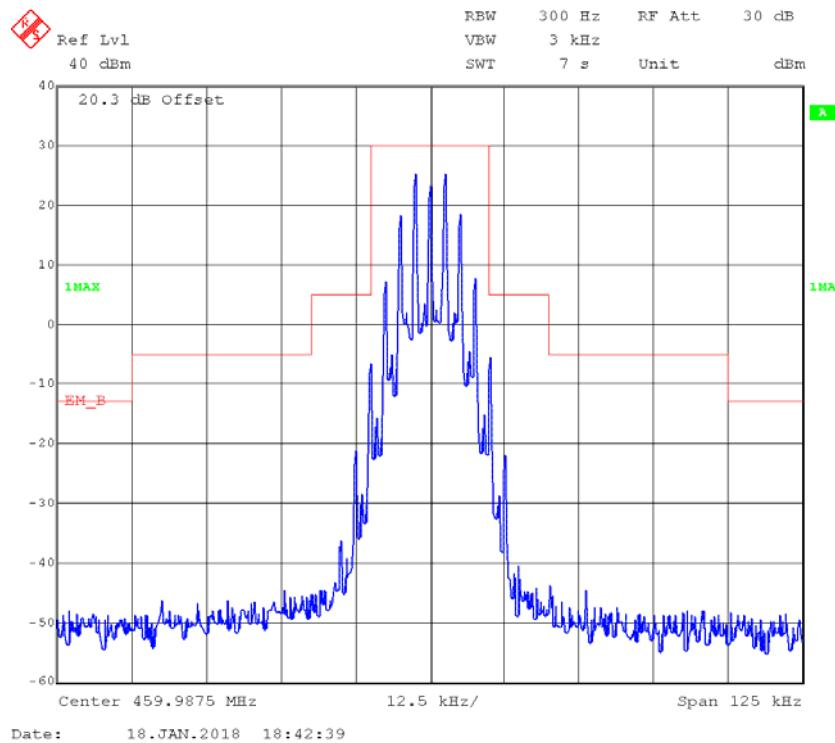
**Part 74****FM,12.5kHz,High Power - Frequency 450.03125 MHz: 99% Occupied & 26 dB Bandwidth**
