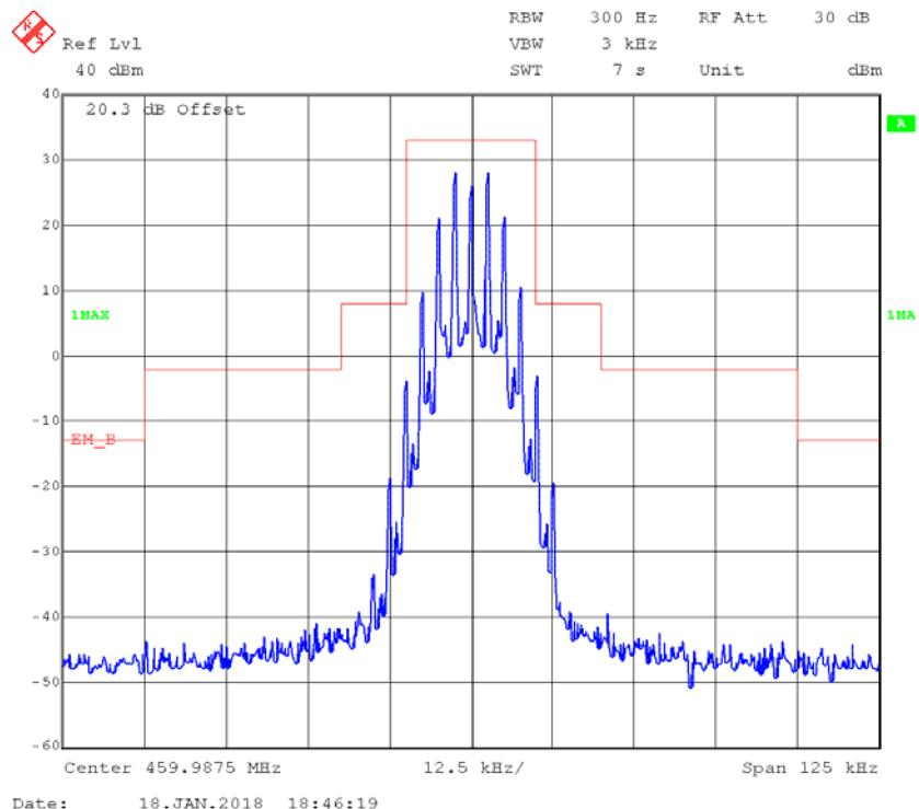
**FM,25kHz,Low Power - Frequency 459.9875 MHz MHz: 99% Occupied & 26 dB Bandwidth**
