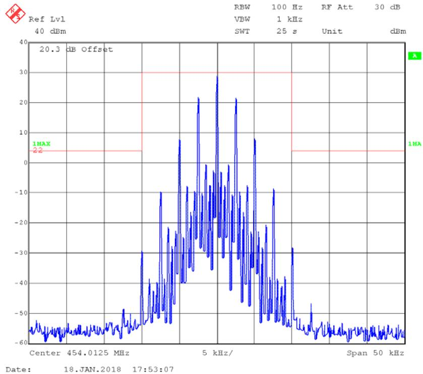
**FM,25kHz,High Power - Frequency 454.0125 MHz: 99% Occupied & 26 dB Bandwidth**
