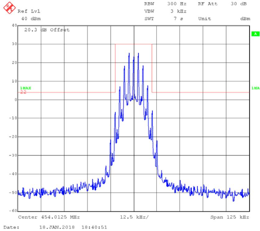
**4FSK,12.5kHz,High Power - Frequency 454.0125 MHz: 99% Occupied & 26 dB Bandwidth**
