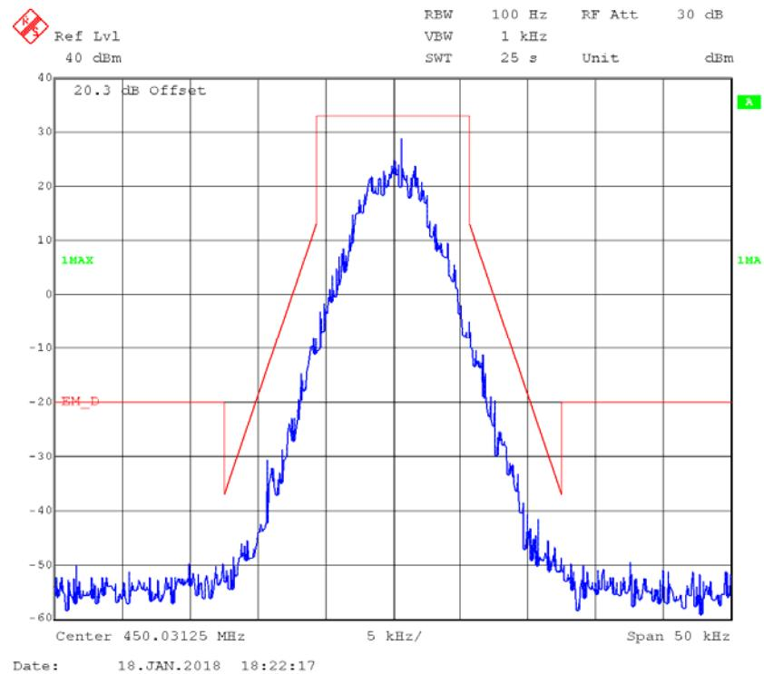
**4FSK,12.5kHz,Low Power - Frequency 450.03125 MHz: 99% Occupied & 26 dB Bandwidth**
