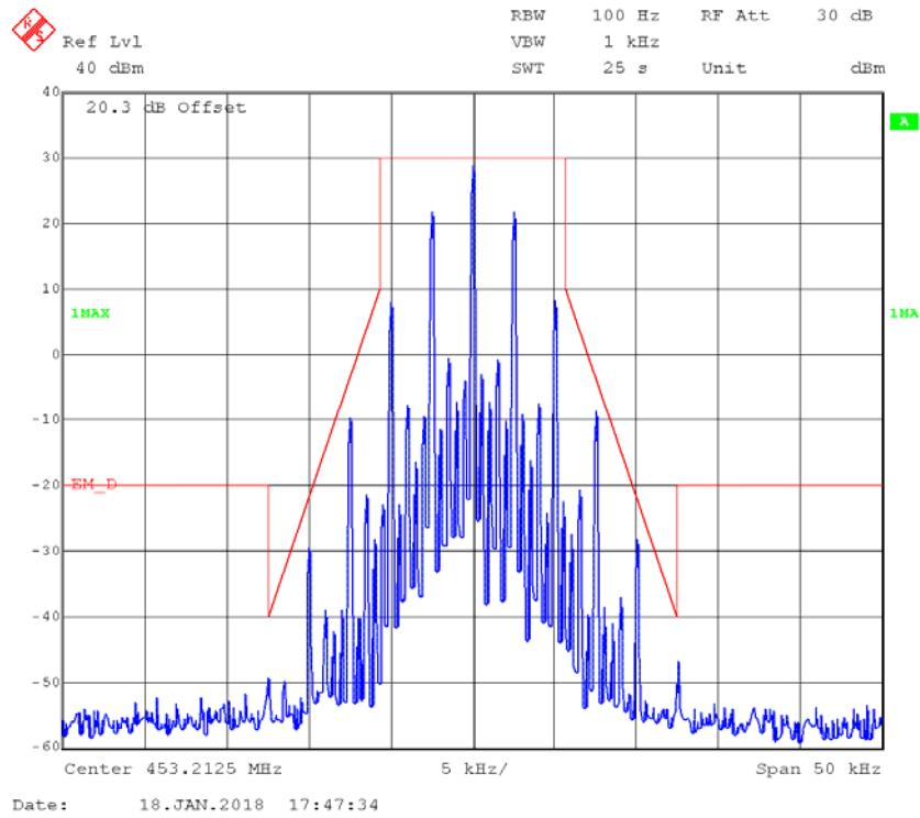
**4FSK,12.5kHz,High Power - Frequency 453.2125 MHz: 99% Occupied & 26 dB Bandwidth**
