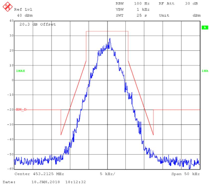
**4FSK,12.5kHz,Low Power - Frequency 453.2125 MHz: 99% Occupied & 26 dB Bandwidth**
