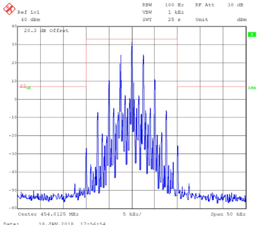
**FM,12.5kHz,Low Power - Frequency 454.0125 MHz: 99% Occupied & 26 dB Bandwidth**
