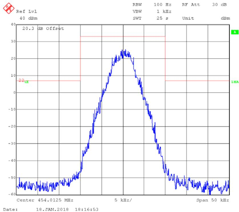
**4FSK,12.5kHz,Low Power - Frequency 454.0125 MHz: 99% Occupied & 26 dB Bandwidth**
