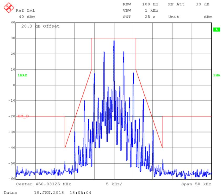
**FM,25kHz,High Power - Frequency 450.03125 MHz: 99% Occupied & 26 dB Bandwidth**
