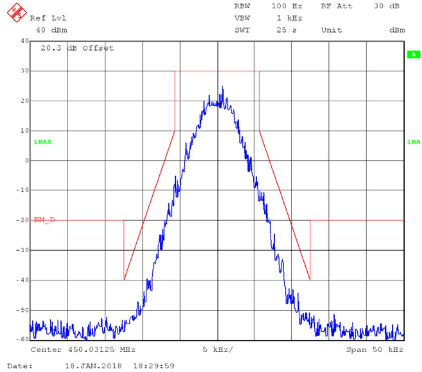
**Part 22****FM,12.5kHz,High Power - Frequency 454.0125 MHz: 99% Occupied & 26 dB Bandwidth**
