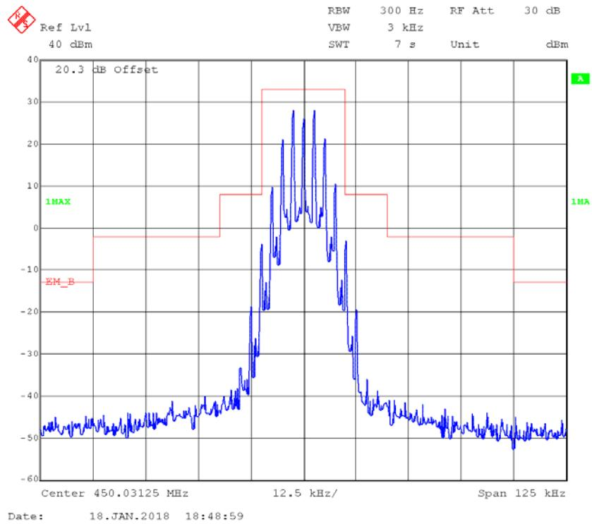
**FM,25kHz,Low Power - Frequency 450.03125 MHz: 99% Occupied & 26 dB Bandwidth**
