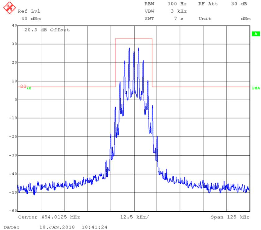
**FM,25kHz,Low Power - Frequency 454.0125 MHz: 99% Occupied & 26 dB Bandwidth**
