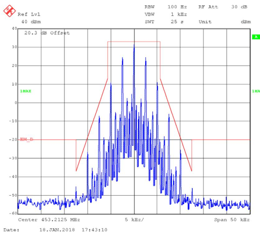
**FM,12.5kHz,Low Power - Frequency 453.2125 MHz: 99% Occupied & 26 dB Bandwidth**
