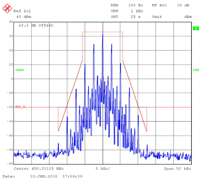
**FM,12.5kHz,Low Power - Frequency 450.03125 MHz: 99% Occupied & 26 dB Bandwidth**
