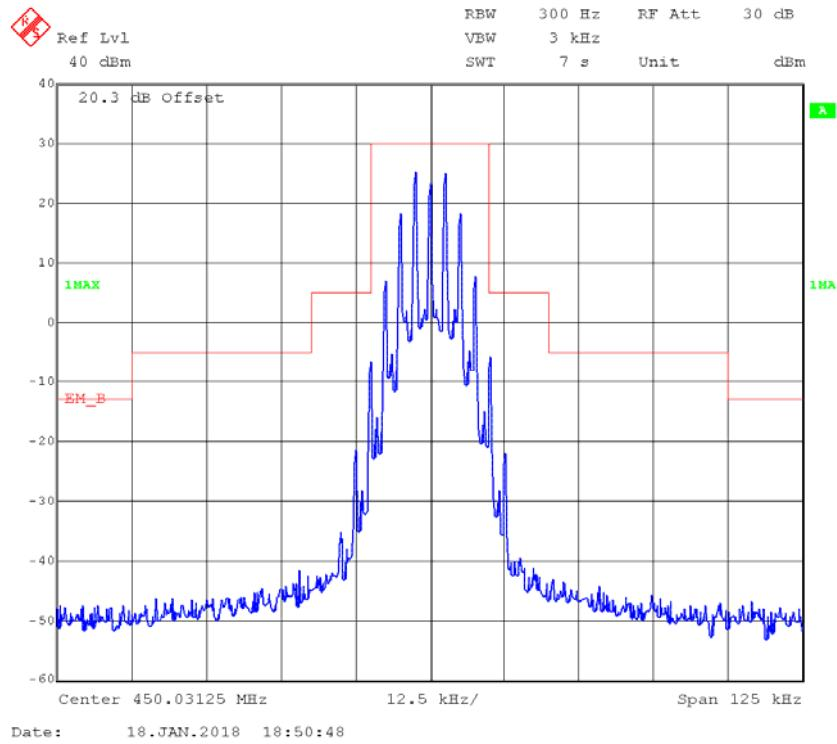
**4FSK,12.5kHz,High Power - Frequency 450.03125 MHz: 99% Occupied & 26 dB Bandwidth**
