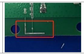
The antenna is PCB antenna. The best case gain of the antenna is 0 dBi.
