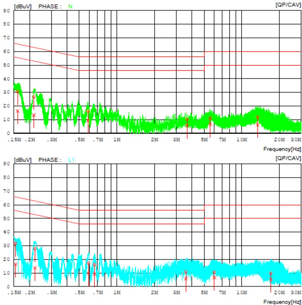
**AC Line Conducted Emissions (List)****AC Line Conducted Emission**
