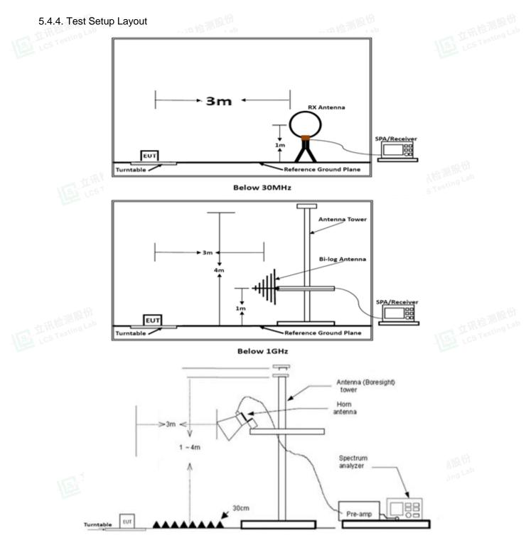
Above 18 GHz shall be extrapolated to the specified distance using an extrapolation factor of 20 dBdecade form 3m to 1m.
