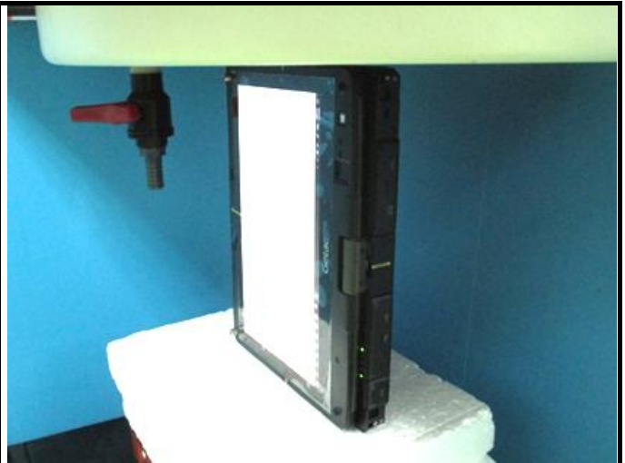
Body - Right Side of EUT at 0 mm
