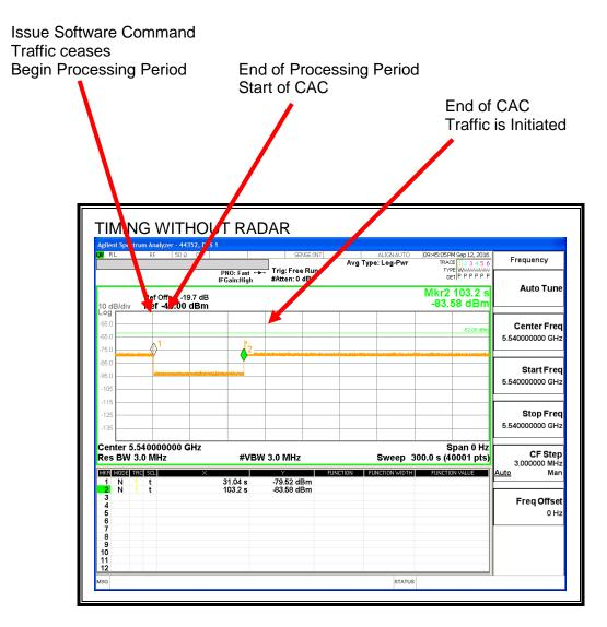
Transmissions begin on channel after completion of the initial processing period and CAC.
