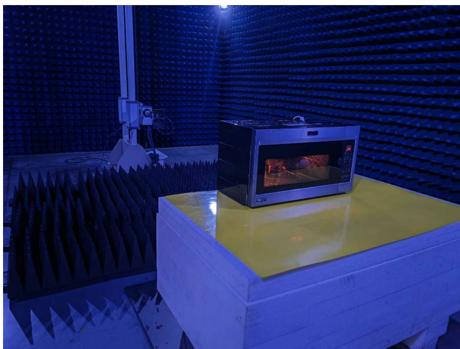
Photo of Radiated Emission Measurement Above 1GHz
