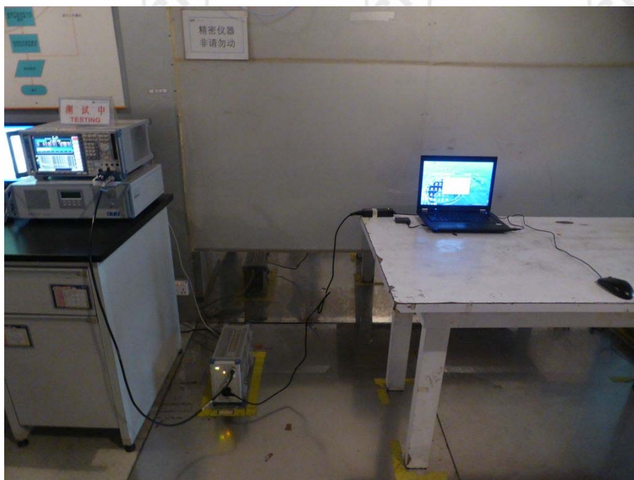
Conducted Emissions Test Setup
