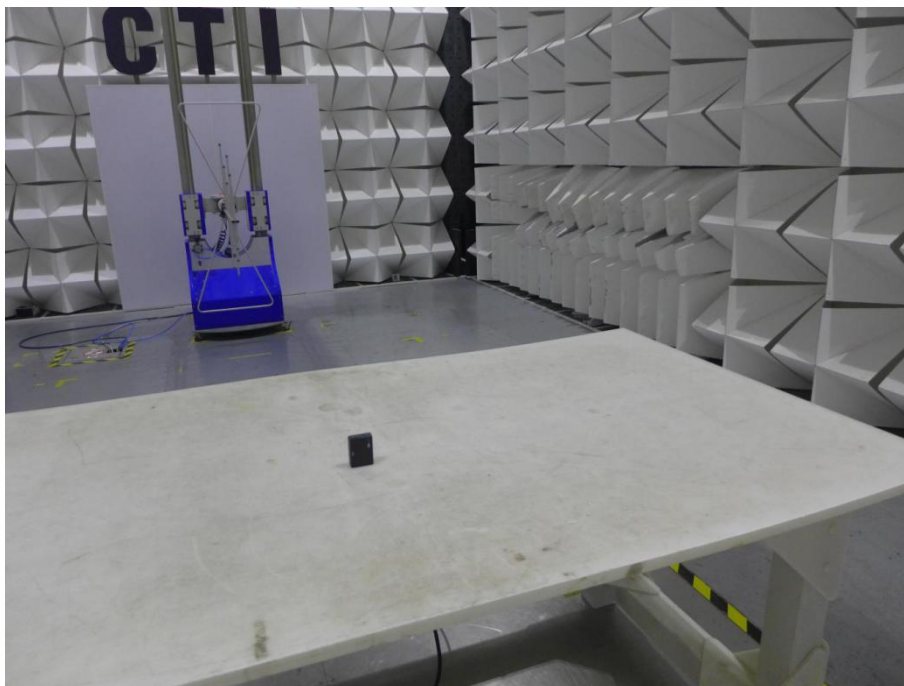
Radiated spurious emission Test Setup-1(Below 1GHz)
