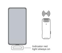
Step 3: The indicator Red light of receiver keeps always on,
