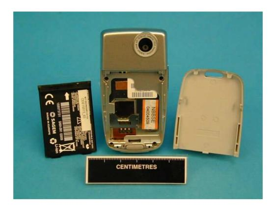
Sagem MC2004a - Rear View (Battery removed)
