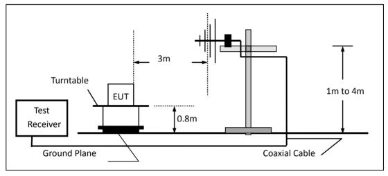
(c) For radiated emissions above 1000MHz
