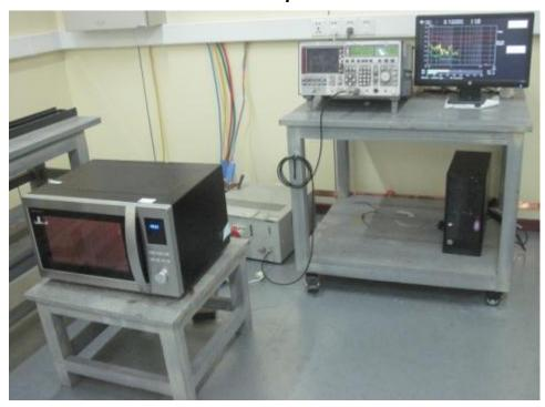
Radiated Emission Test Set-up (30 -1,000MHz):
