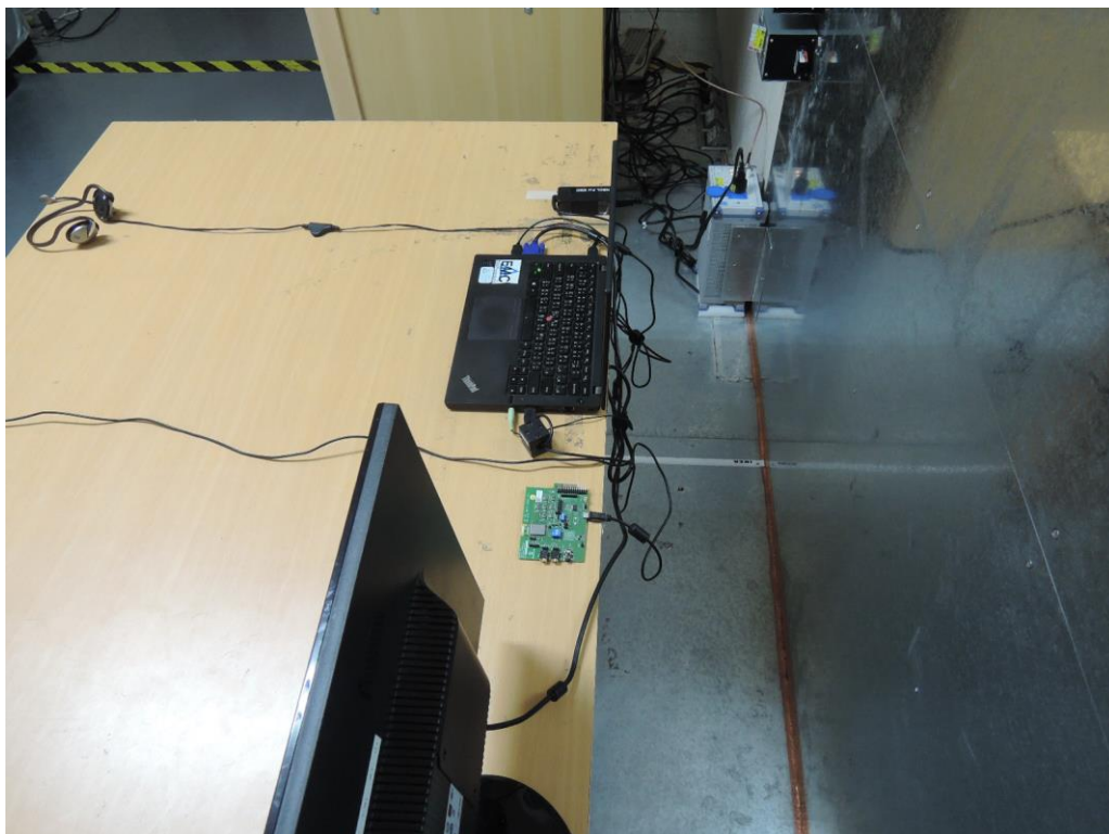
Photograph 5: Set-up for for Mains Conducted testing Back
