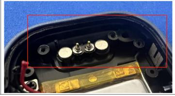
The antenna is Metal frame antenna.
