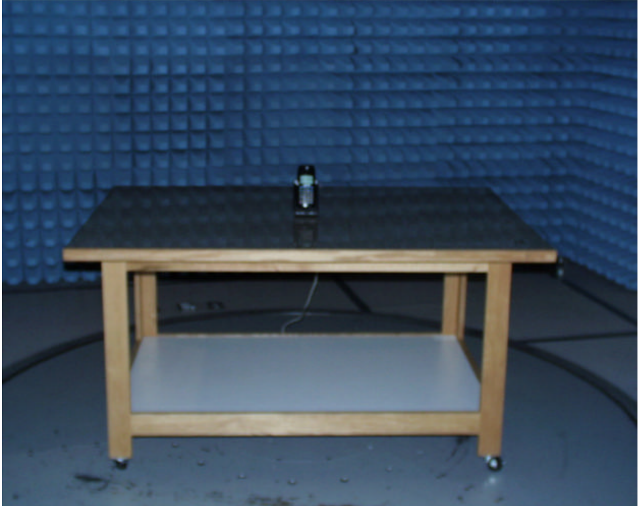
Front View of Worst Case Radiated Emissions
