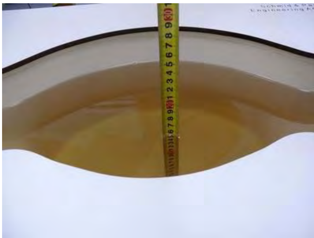
Picture 4: Liquid depth in the flat Phantom (835MHz, 15.4cm depth)
