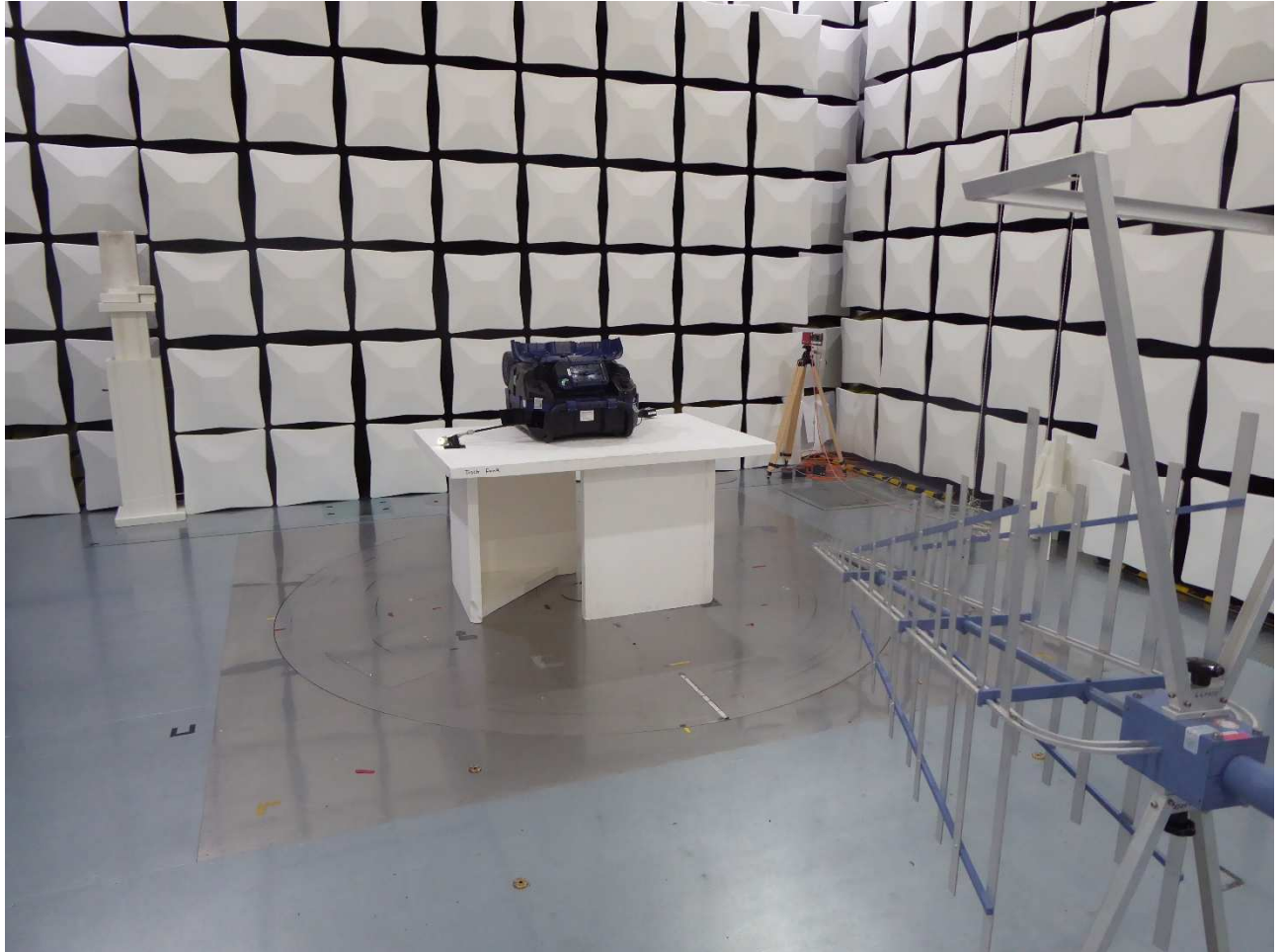
Test setup semi anechoic chamber (30 MHz – 1 GHz)
