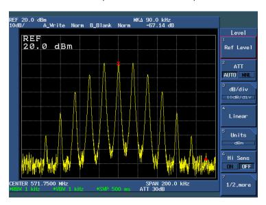
OCCUPIED BANDWIDTH—POWER OUTPUT = 250 Watts Visual 25 Watts Aural (Scan width = 200 kHz)
