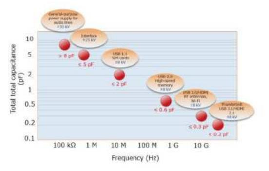
Figure 4.7 TVS diode junction capacitance selection reference
