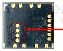
In the **5.6\*1.5mm** area of the upper left corner of the module BOTTOM layer, there are 4 test point pads with windows and exposed copper. It is best not to go to the position mapped to the bottom plate area.
