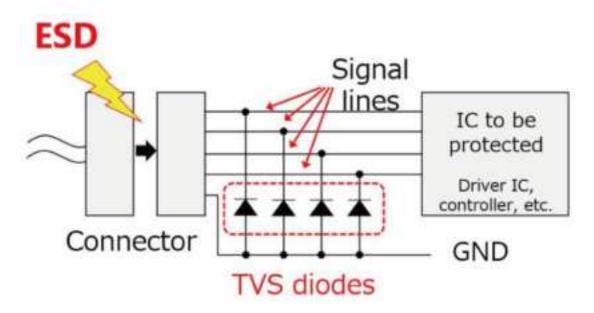
Figure 4.5 TVS diode protection IC
