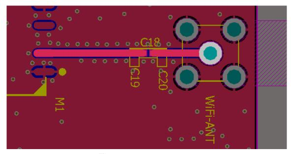
Figure 5.3 The impedance line of the base plate
