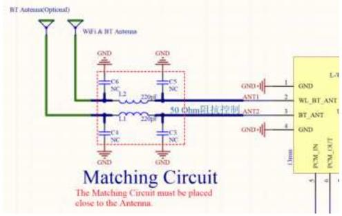
Figure 5.2 RF interface and matching circuit design reference
