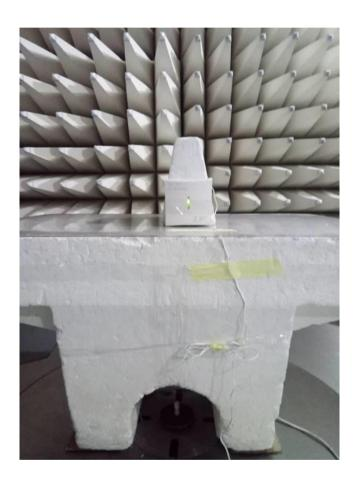
Photograph No.5 Setup for 20 dB bandwidth measurements
