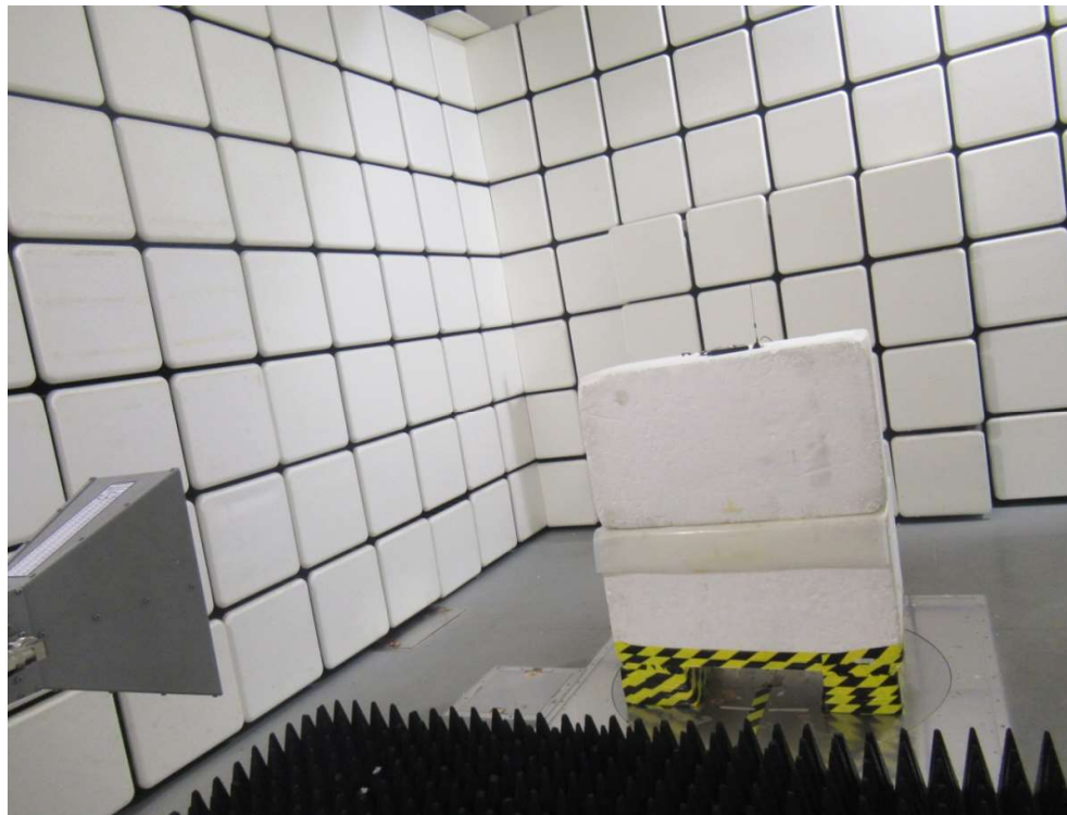
Picture 1: Radiated Spurious Emissions Test setup
