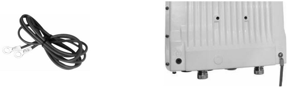
Figure 3-24 Ground the device
