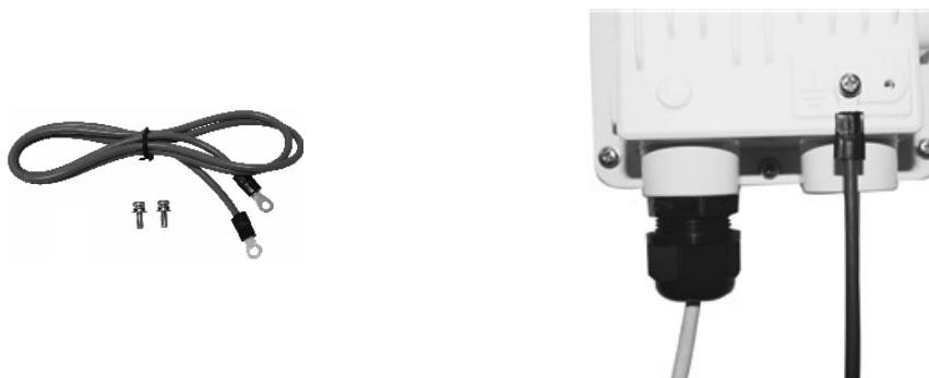
Figure 2-18 Ground the Device
