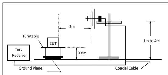
(c) For radiated emissions above 1000MHz
