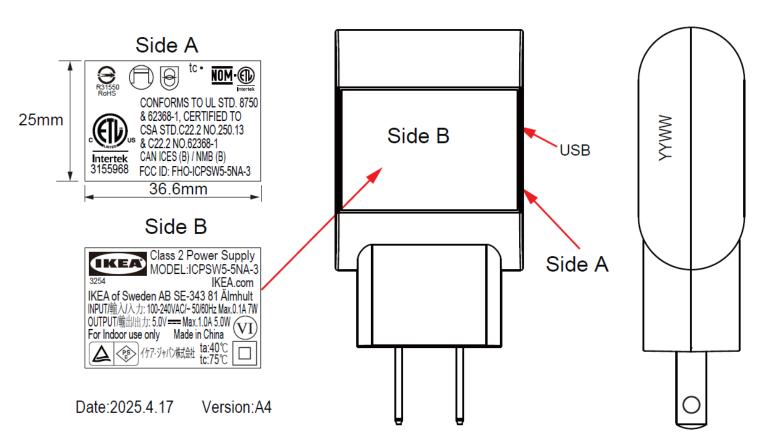
Manufacturing date "YYWW" will be attached separately on the product according to position marked YYWW. "YY" representing year of manufacturing (e.g. year 2019 is shown as "19")
