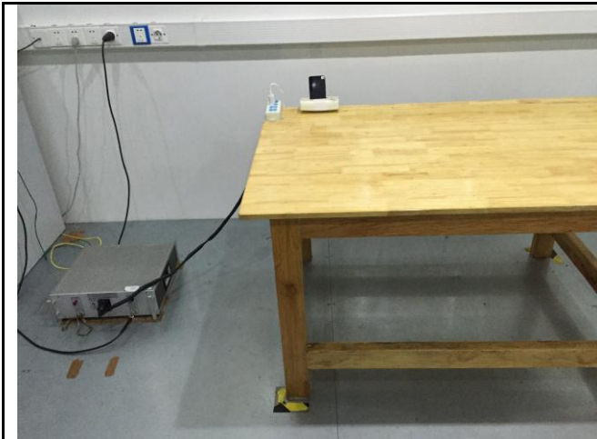
Conducted Emissions Test Setup Front View
