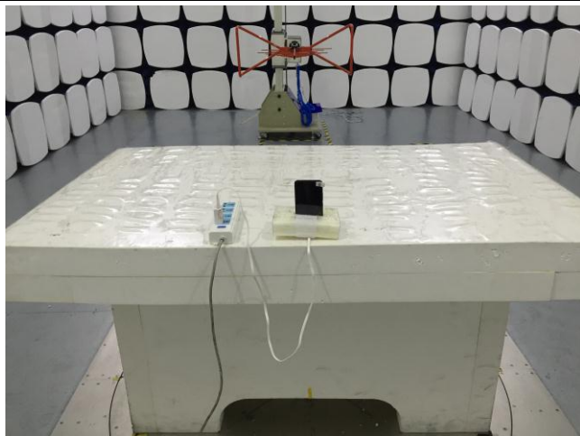
Conducted Emissions Test Setup Front View
