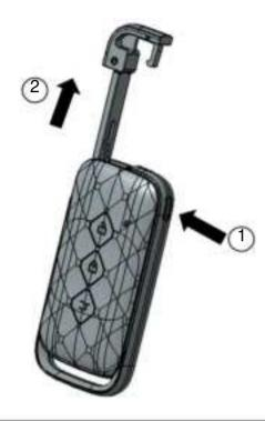
As shown in the figure above, first press the release switch ① on the key, and then pull out the mechanical key ②, After use, insert the mechanical key back.
