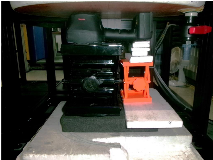
Figure D.5: DUT back face touching the body at 0mm gap configuration.
