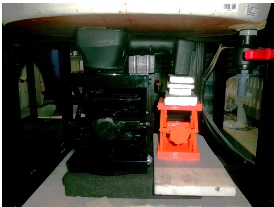
Figure D.4: DUT front face touching the body at 0mm gap configuration.
