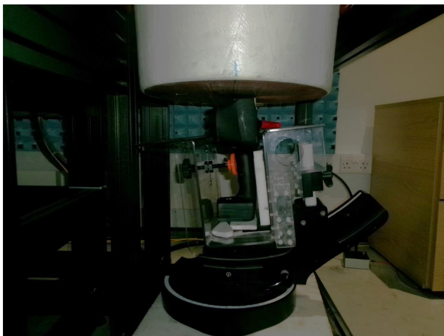
Figure D.6: DUT top face touching the body at 0mm gap configuration.
