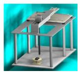
**Figure 4-3** RF Near-Field Scanner
