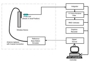
Figure 4-13 **Audio Magnetic Field Test Setup**
