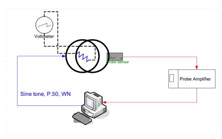
Figure 4-1 Validation Setup with Helmholtz Coil
