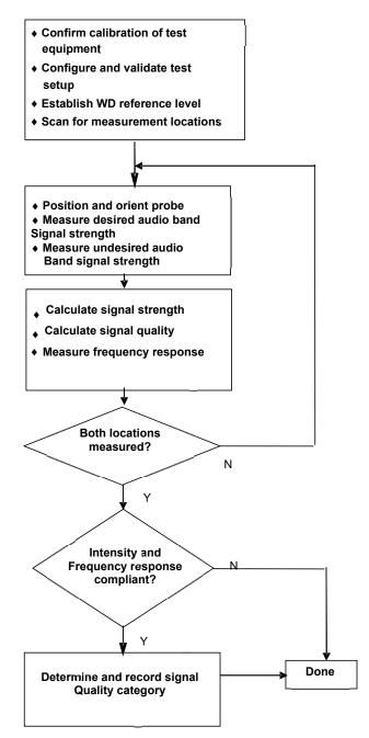
Figure 4-14 C63.19 T-Coil Signal Test Process
