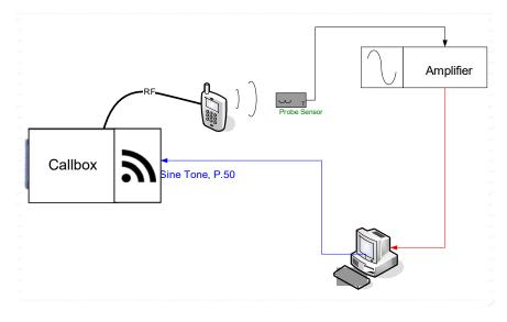
Figure 4-2 **T-Coil Test Setup**
