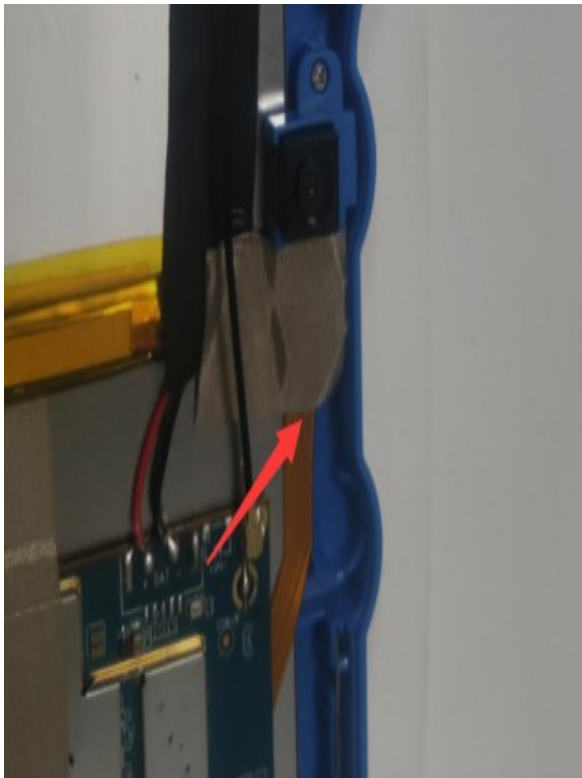
Camera cable is shielded by conductive cloth
