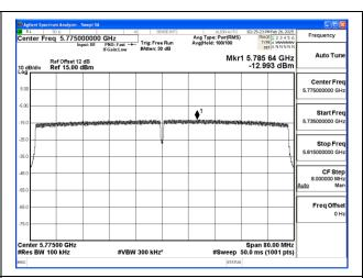
Mode:802.11ac VHT80 Frequency:5775MHz
