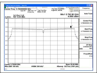
Mode:802.11ac VHT20 Frequency:5745MHz
