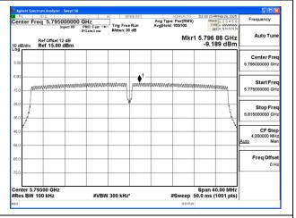
Mode:802.11ac VHT40 Frequency:5755MHz
