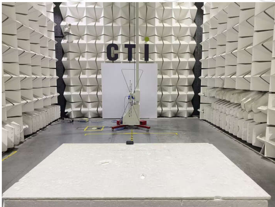
Radiated spurious emission Test Setup-1(Below 1GHz)
