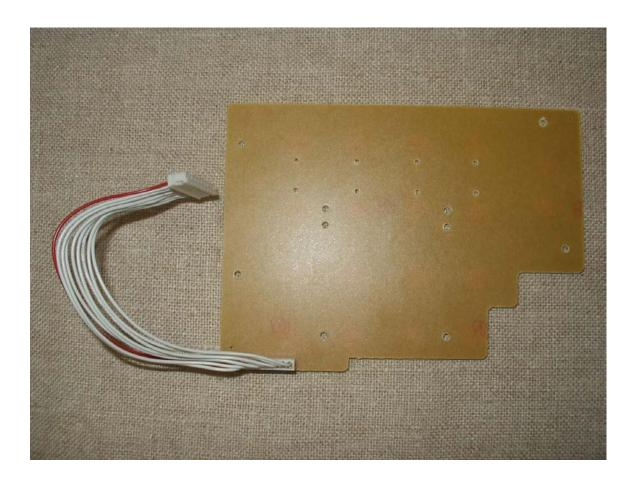
Figure 1-2: Internal photograph, Keypad PCB (bottom)
