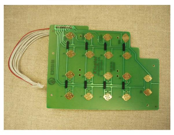
Figure 1-1: Internal photograph, Keypad PCB (top)
