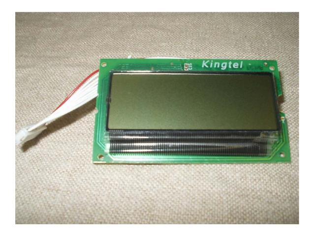
Figure 1-3: Internal photograph, LCD PCB (top)
