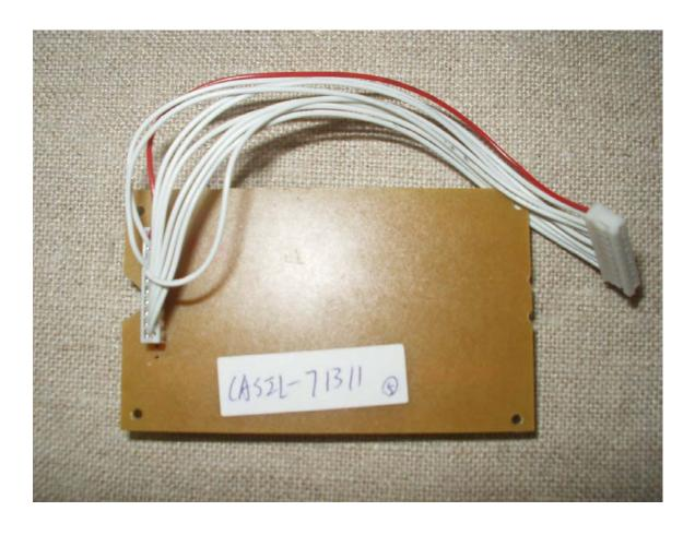
Figure 1-4: Internal photograph, LCD PCB (bottom)
